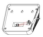
3. Connect audio cable to the Phoenix connector located on the rear panel. Power taps for both loudspeaker models are marked near the connector.
