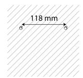
1. Fix mounting screws on solid surface (recomended distance between centers of screws holes is 118 mm for both models).
