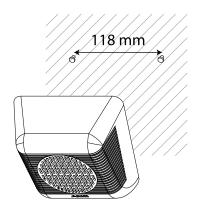
4. Fix the loudspeaker on the wall.
