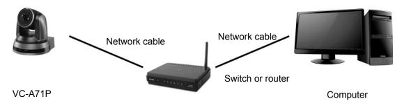
2. To connect directly through network cable, the IP address of the computer should be changed so that it is on the same network segment as the camera e.g.: The factory-preset default IP address of VC-A71P is 192.168.100.100. The computer IP address must be set with the same network segment, such as 192.168.100.101, so that the computer can be connected correctly with the camera
