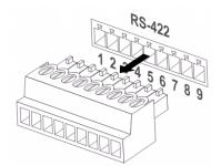
2. Peel off a section of copper wire (AWG Nos. 28 to 18) and insert it into the connector hole; then use flat screw driver to fix it
