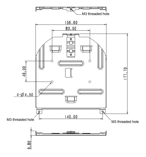
Metal plate A - machine side
